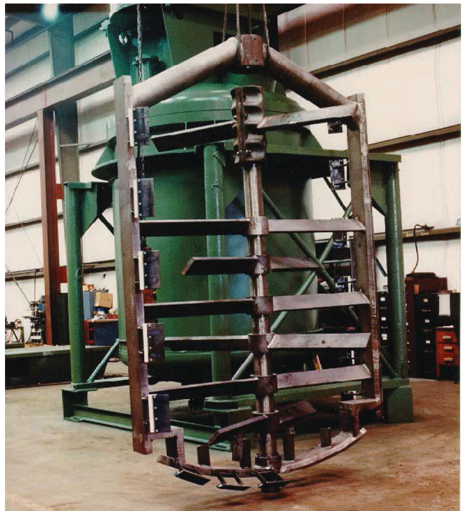
Figure 2 | Agitator blades (horizontal) and scrapers (white vertical rectangles). (Figure courtesy of CITGO Petroleum Corp.)
